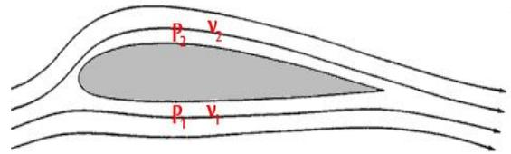
Figure 1 - the change in streamlines around an aerofoil.
